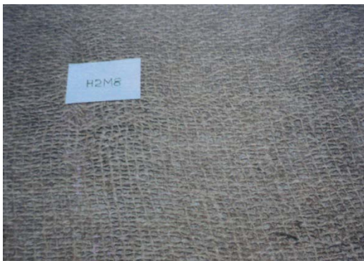
Woven coir netting / Mesh matting used as geotextiles
